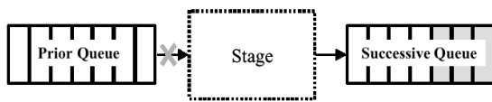
Figure 20: The stage cannot be active since the prior queue is empty. After the prior stage produces results, the current stage can continue its job.
