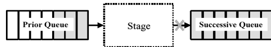
Figure 22: The stage cannot be active since the successive queue is full. The stage can continue its job after the successive stage consumes some data from the successive queue.
