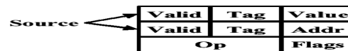
Figure 15: The structure of one LSQ element. The address field is the result of the additional address computation operation.
