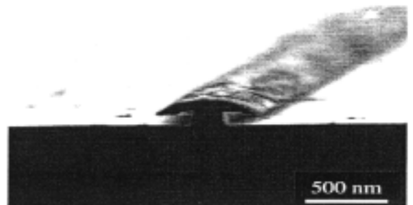
Fig.2 SEM of the T-shaped gate.
