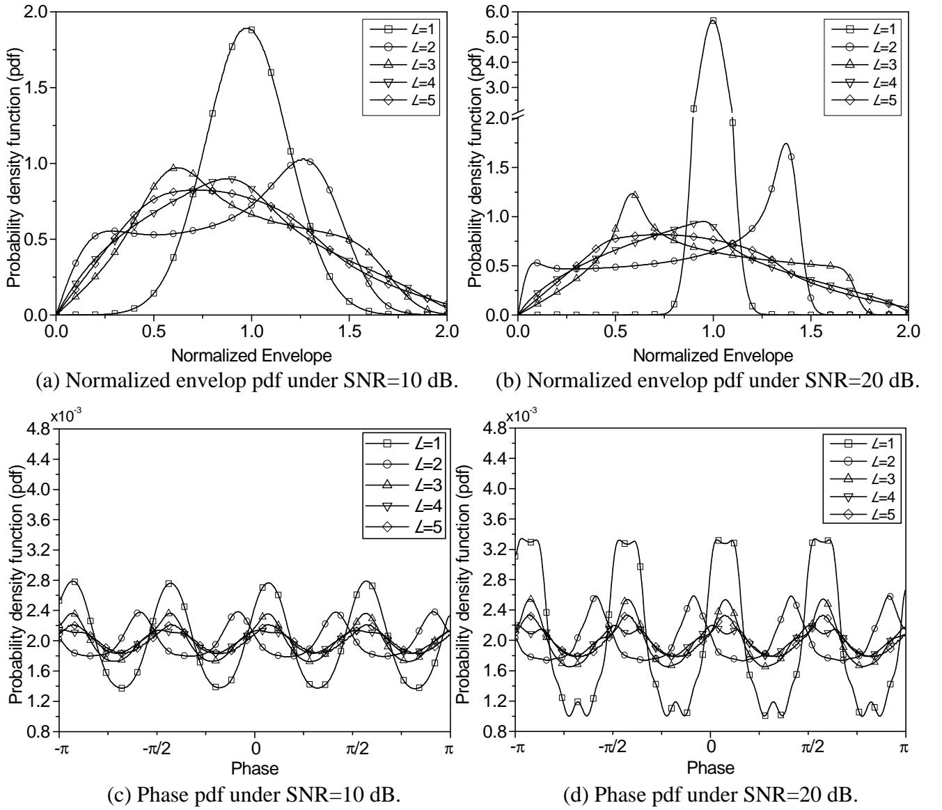
Figure 4. Envelope/phase pdf's under different  $L$ 's.
