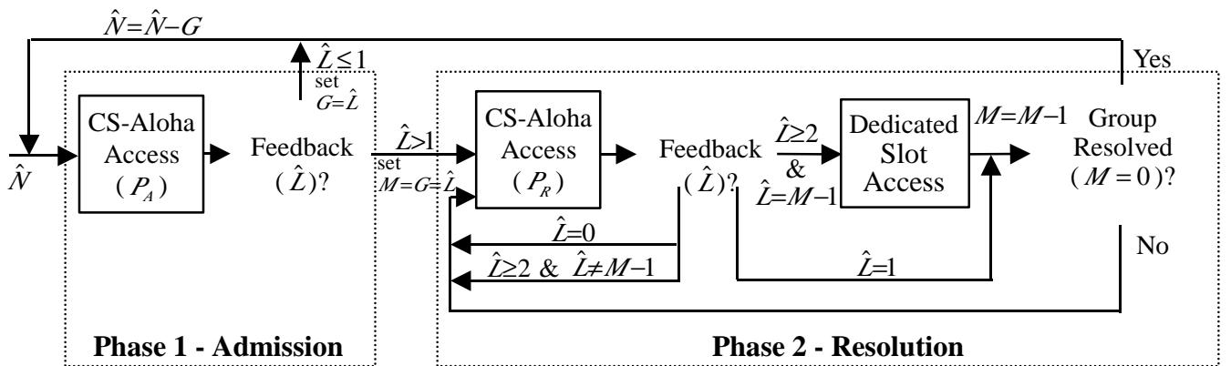
Figure 2. Two-phase process of HFCA.
