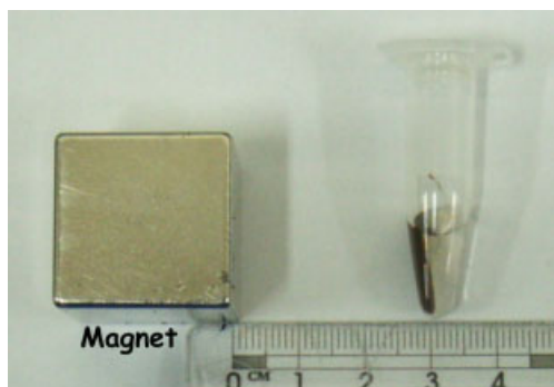
Figure 5. Photograph showing a magnet placed at a distance within 3 cm of the vial containing bacteria and magnetic nanoparticles.
