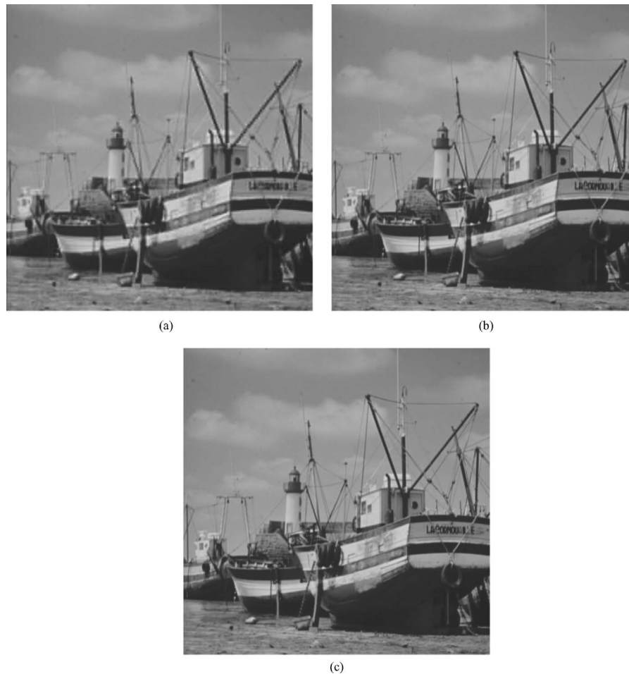
Fig. 7 The reconstructed Boat image of (a) low, (b) low+middle, and (c) low+middle+high frequencies. The PSNRs are 28.18, 32.83, and 37.64 dB, respectively. Note that (a) is from any 3 of the 6 images in Fig. 6(b1')–(b6'); (b) is from any 4; and (c) is from any 5.
