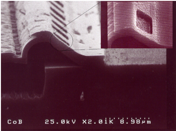
Fig. 3. The etching holes were already been uniformly filled with aluminum layer and no gap is observed.
