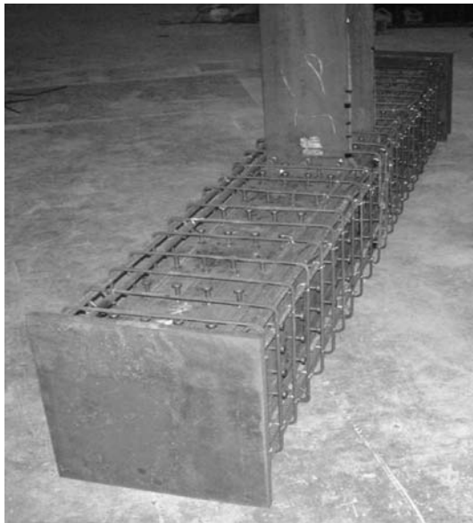
Photo 2 Specimen SRC2-BOX-S in preparation
