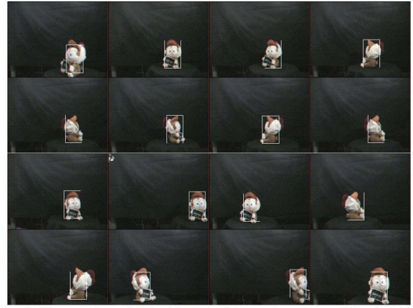
Fig. 4. The results of 3D object tracking using mean-shift algorithm without 3D object database, where frame 76, 141, 205, 341, 373, 437, 469, 509, 733, 805, 885, 965, 990, 1095, 1135, 1261 are listed from left to right and from top to down.
