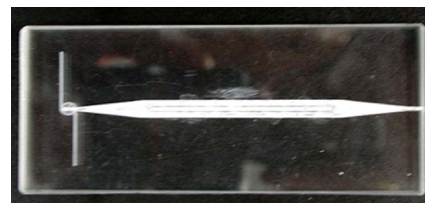
FIG. 3. (Color online) Optical microscope image of the fluidic system with the straight channels immobilized LDHs for extraction of DNA molecules. The helixlike structure at left side was the injected inlet for sample solution.
