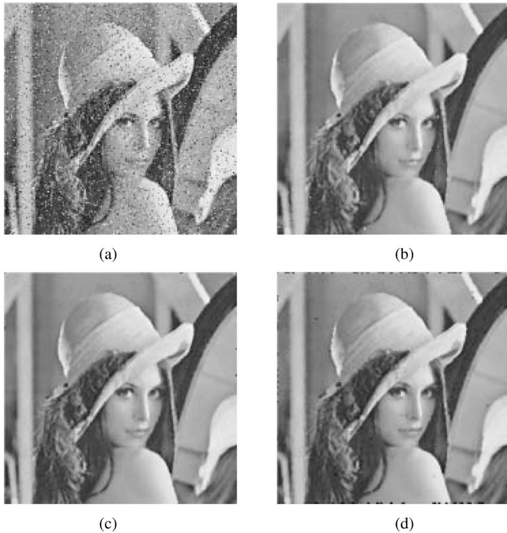
Fig. 27. Simulation results of a 2-D ROF application. (a) The noisy “Lena” image corrupted by 8% of impulsive noise. (b) The “Lena” image processed by the 3 \times 3 4th-order filtering. (c) The “Lena” image processed by the 3 \times 3 5th-order filtering. (d) The “Lena” image processed by the 3 \times 3 6th-order filtering.
