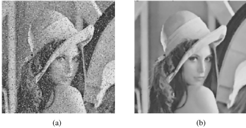
Fig. 28. Simulation results of a 2-D RMF application. (a) The noisy “Lena” image corrupted by 9% of impulsive noise. (b) The “Lena” image processed by the 3 \times 3 RMF.
