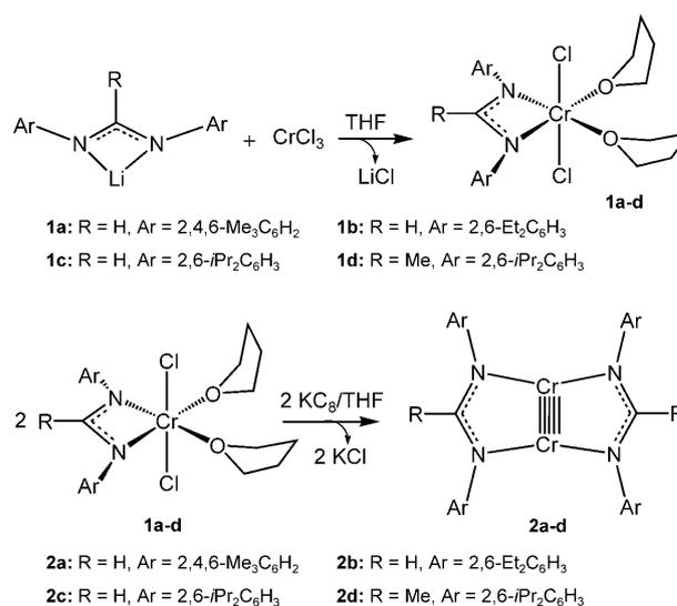
**Scheme 1.** Synthesis of complexes [CrCl<sub>2</sub>(thf)<sub>2</sub>{ $\eta^2$ -ArNC(R)NAr}] (**1a–d**) and [Cr<sub>2</sub>{ $\mu$ - $\eta^2$ -ArNC(R)NAr}]<sub>2</sub> (**2a–d**).
