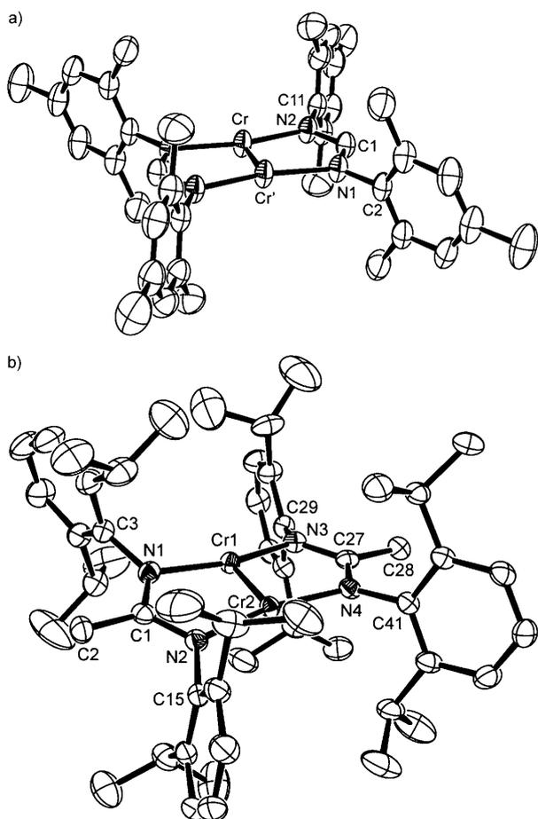
**Figure 1.** Molecular structures of **2a** (a) and **2d** (b) with thermal ellipsoids set at 30% probability. Hydrogen atoms have been omitted for clarity.
