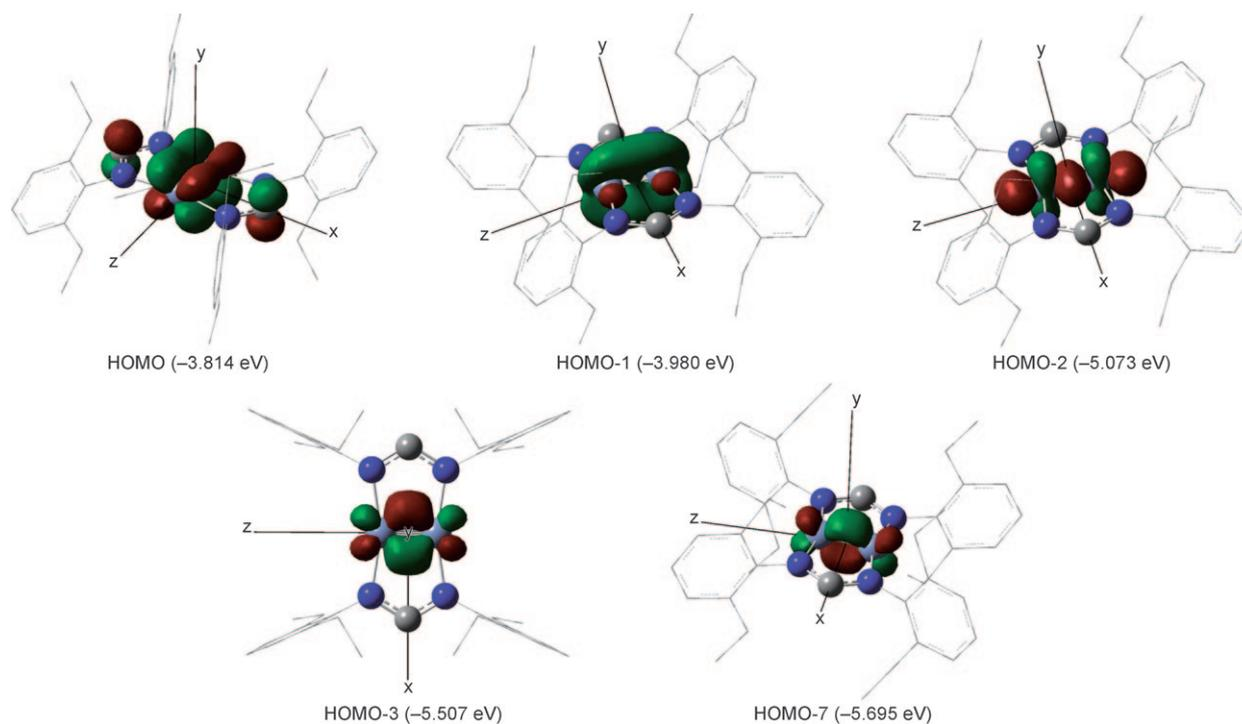
**Figure 3.** Frontier orbitals displaying Cr–Cr bonding in **2b**.
