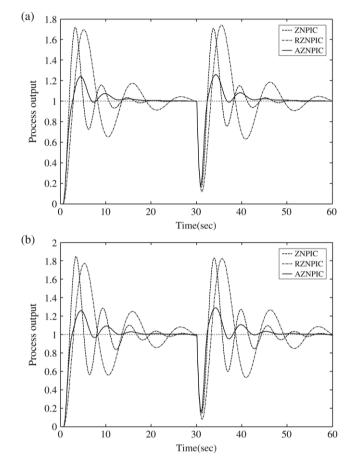
Fig. 7. Responses of the third-order linear process in (14) with (a)  $L=0.4~{\rm s}$  and (b)  $L=0.5~{\rm s}$ .
