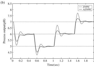
Fig. 9. Responses of pH process in (16) with  $L=0.02\,\mathrm{s}$  for (a) both set-point change and load disturbance and (b) set-point change from different operating points.
