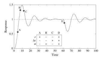
Fig. 3. Typical close-loop response of an under-damped second-order process.
