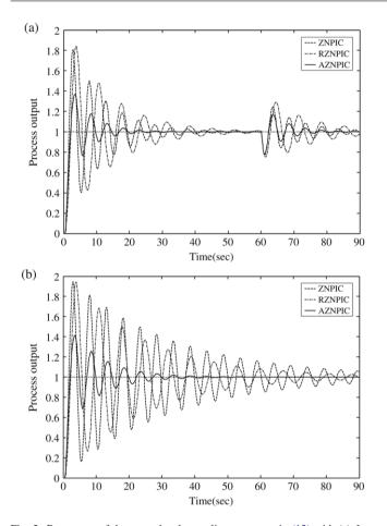
Fig. 5. Responses of the second-order nonlinear process in (12) with (a)  $L=0.2\,\mathrm{s}$  and (b)  $L=0.3\,\mathrm{s}$ .
