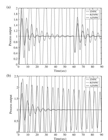
Fig. 6. Responses of the marginally stable process in (13) with (a)  $L=0.2~{\rm s}$  and (b)  $L=0.3~{\rm s}$ .
