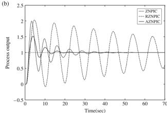
Fig. 8. Responses of the third-order nonlinear process in (15) with (a)  $L=0.3\,\mathrm{s}$  and (b)  $L=0.4\,\mathrm{s}$ .
