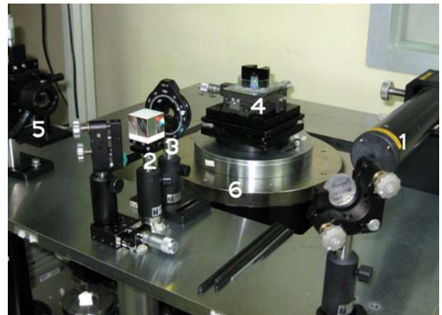
Figure 3. A laser diffractometer assembled on the precision rotating table.
