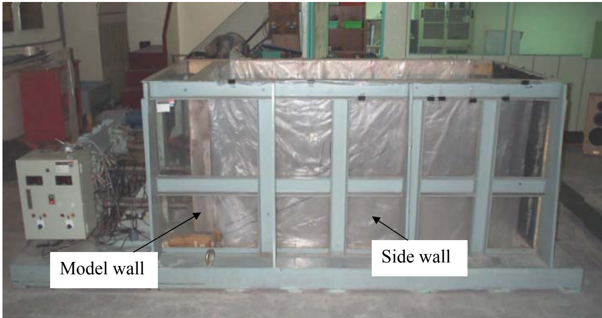
Fig. 10. Picture of NCTU model retaining wall
