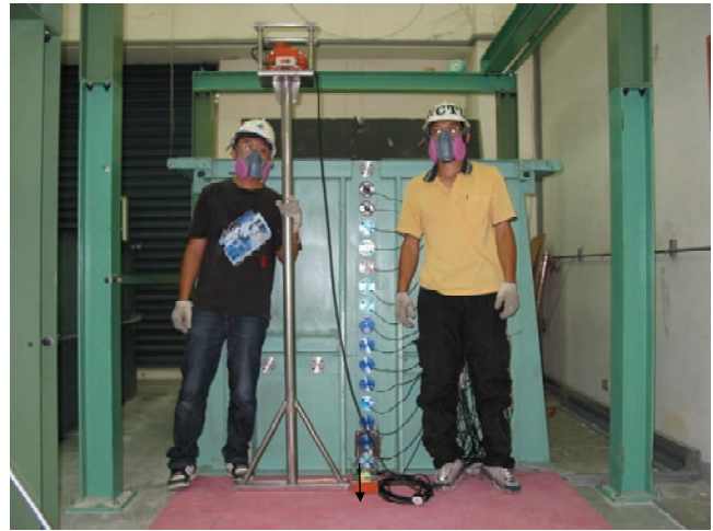
Fig. 4. Strip vibratory soil compactor and model wall
