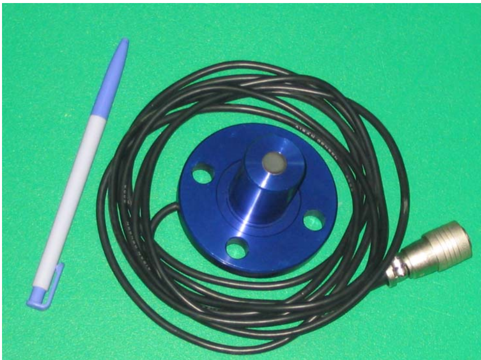
Fig. 11. Soil pressure transducer (Kyowa PGM-0.2KG)
