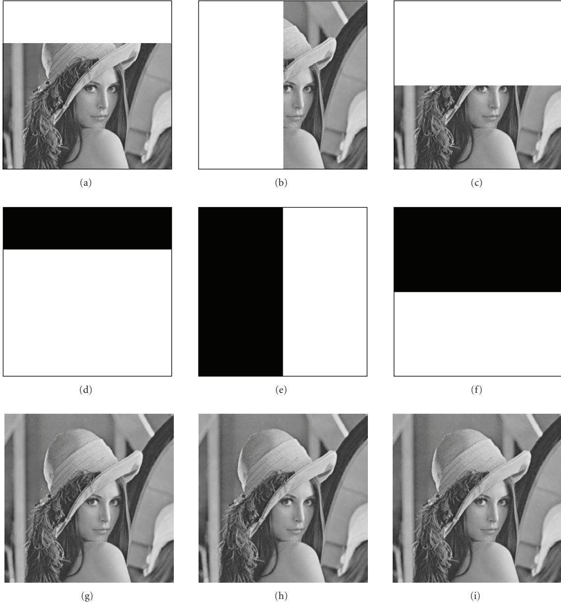
FIGURE 6: The cropping attack experiments: (a) 25% of the watermarked image Lena (W) is cropped; (b) a vertical cropping of 50%; (c) a horizontal cropping of 50%; (d)–(f) the detected tampered blocks of (a)–(c), respectively; (g)–(i) the images recovered from (a)–(c), respectively. The PSNR values are 40.04 dB for (g); 34.77 dB for (h); and 36.54 dB for (i).
