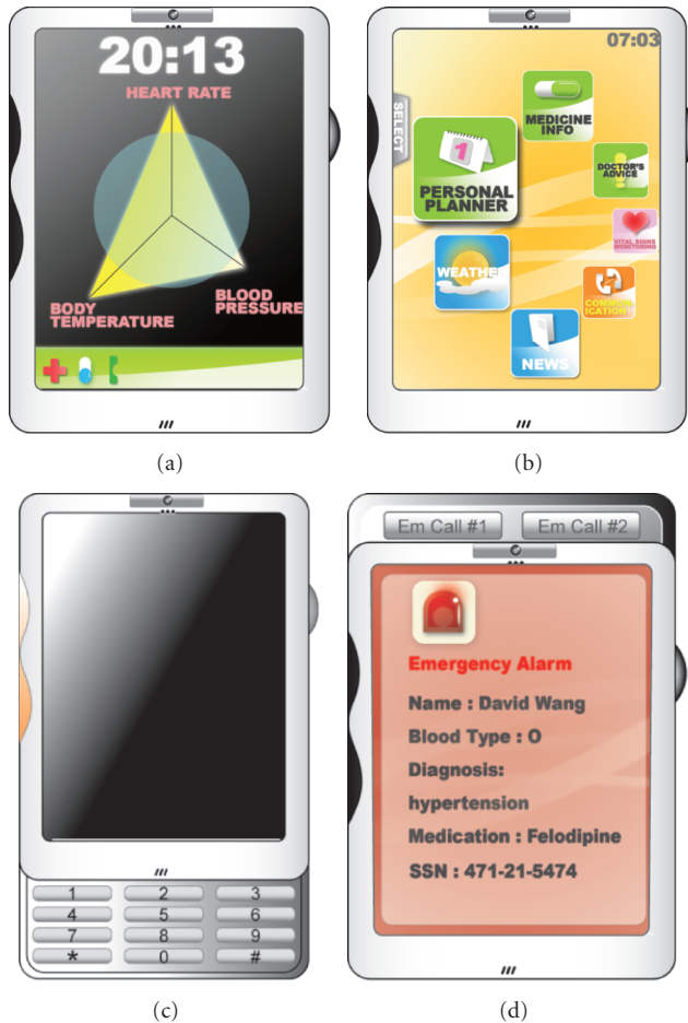
FIGURE 5: (a) Screen saver, (b) main menu, (c) pull-down keypad, (d) pull-up emergency calling pad.
