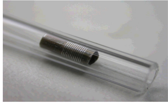
Figure 4. A flexible CMOS wafer piece ( \sim 1.2 cm × 1.2 cm) curled into a cylindrical shape and inserted into a 4 mm diameter glass capillary tube.
