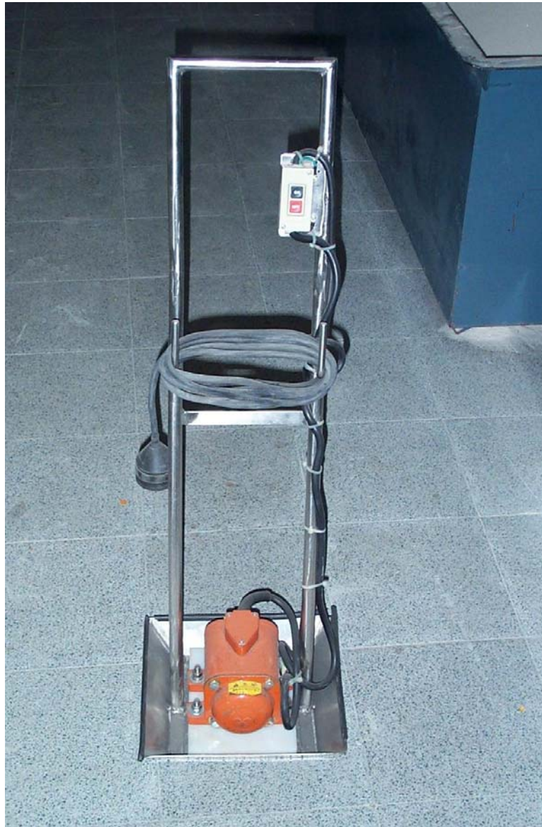
Fig. 9. Vibratory soil compactor (after Chen, 2002)
