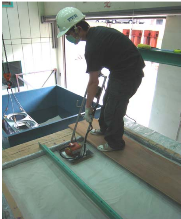
Fig. 1. Compaction of sand with a vibratory compactor
