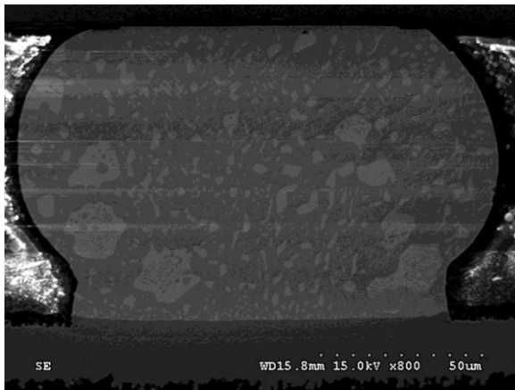
Fig. 5. Cross-sectional SEM images of the as-received sample.
