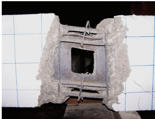
Figure 6 Shear deformation of the steel web of specimen S4
