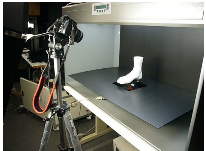
Fig. 6. The hardware setup of the multi-view capturing system with a turntable connected to a PC.
