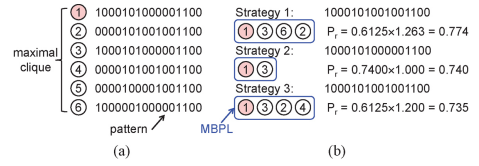
Fig. 5. Clock gating strategies. (a) Clock gating patterns of a maximal clique {1, 2, 3, 4, 5, 6}, where pulsed-latch 1 is essential. (b) The results of Strategies 1, 2, 3 using the MBPL library given in Table I.
