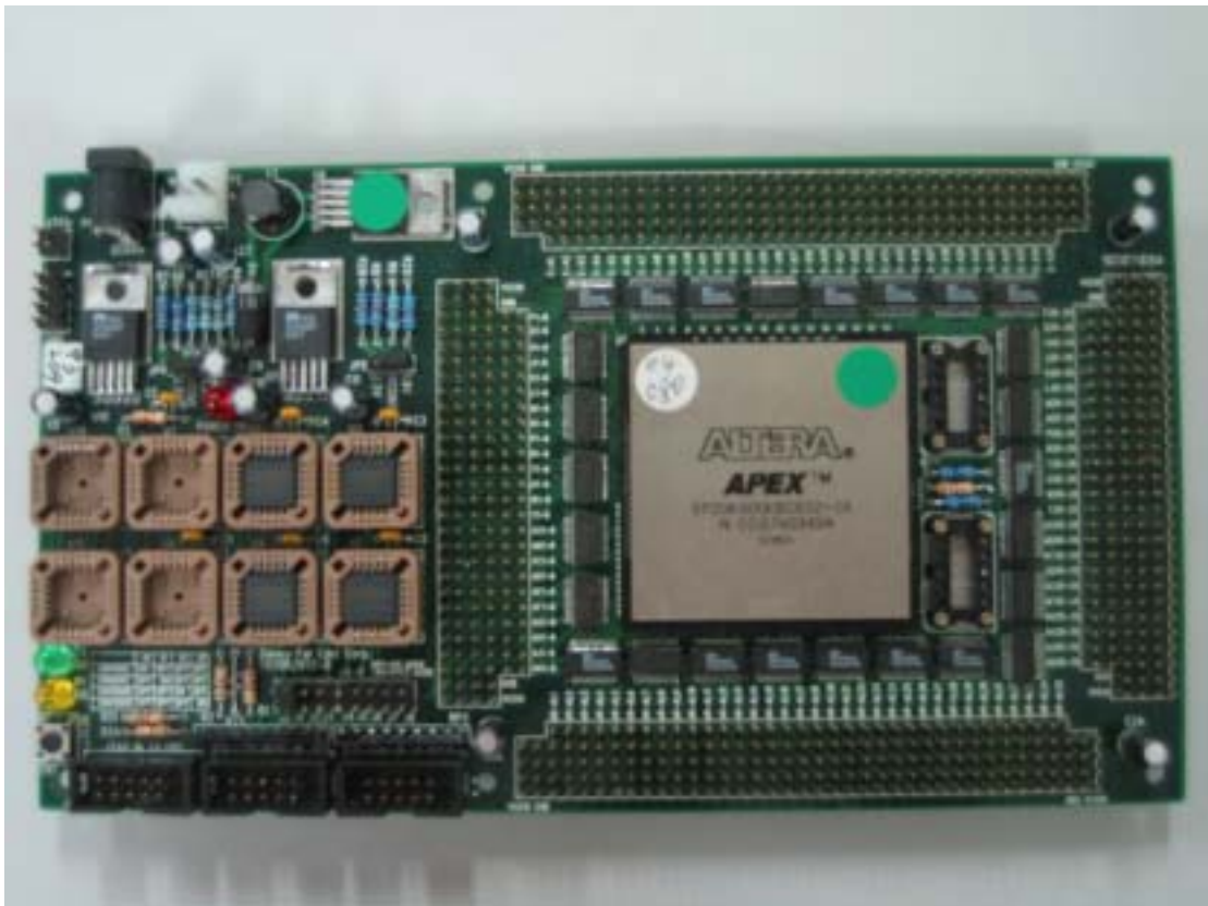
Fig. 9 ALTERA APEX 20KE Family BGA 652 PIN Emulation Board
